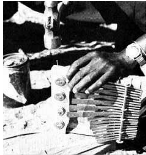
20. THE BOTTLE-TOP BUZZING MECHANISM IS NAILED TO THE SOUNDBOARD
