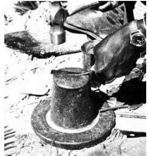
18. A FINISHED KEY IS BENT AT THE POINT WHERE THE TAIL AND THE SPATULATE PORTION MEET
