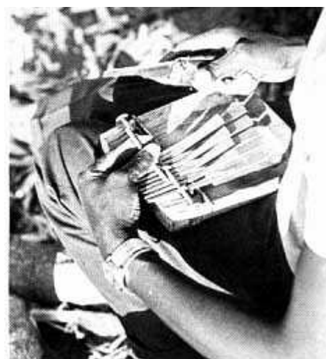
15. FINISHED KEYS ARE ADJUSTED ON THE SOUNDBOARD SO THAT THERE IS AMPLE SPACE
