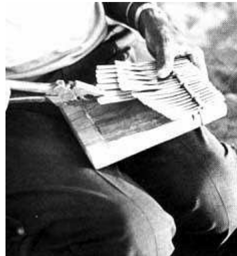
14. THE ENDS OF THE KEYS ARE ADJUSTED SO THAT THEY FORM A STRAIGHT LINE ON EACH MANUAL
